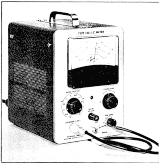
Fig. 2-5. Unmounted capacitor measurement using P93C Probe.
