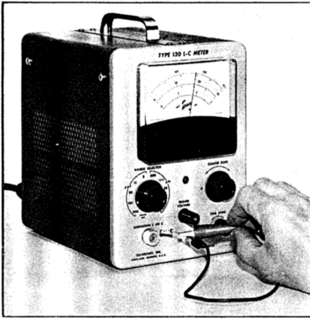
Fig. 2-7. Unmounted capacitor measurement using clip lead.
